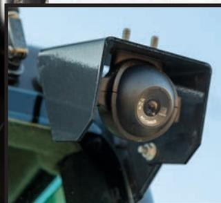
The optional rear camera offers a continuous rear view from the operator's seat, if desired. It helps identify obstacles that, if not avoided, could damage the excavator and its components. The optional camera is mounted high and out of the way to prevent contact with obstacles and debris. A protective structure further ensures rear display reliability.
