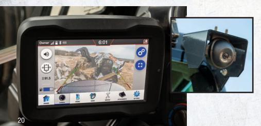
The optional rear camera offers a continuous rear view from the operator's seat, if desired. It helps identify obstacles that, if not avoided, could damage the excavator and its components. The optional camera is mounted high and out of the way to prevent contact with obstacles and debris. A protective structure further ensures rear display reliability.
