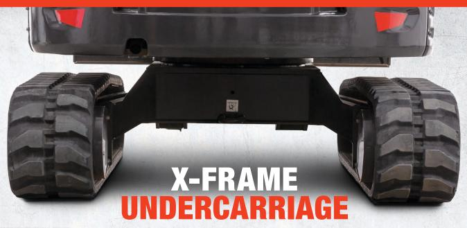
The X-frame design offers increased ground clearance that allows you to go through more. The design sheds debris to reduce your cleanup time as well.
